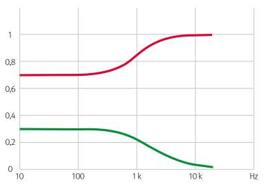
Frequency corrected time difference at max. Crossfeed and 30° Angle of the right channel (red = right signal, green = left signal)
