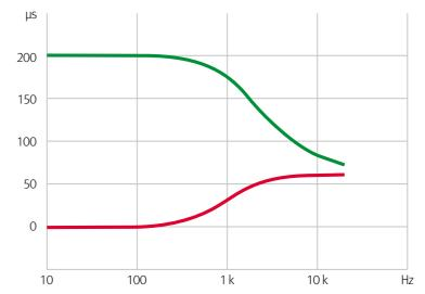
The interaural level difference and the interaural time difference are frequency-corrected because the sound is reflected and absorbed by the head in a non-linear fashion.
