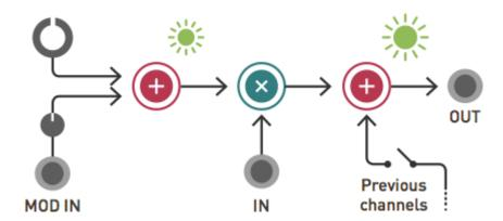
Blinds is a 4-channel voltage-controlled signal polarizer. Each channel consists of a polarizer circuit, also known as a four-quadrant multiplier. This circuit acts like a VCA, except that a negative control voltage will cause the output signal to be inverted, instead of being silenced. Blinds' outputs are daisy-chained, allowing adjacent groups of 2, 3, or all 4 channels, to be mixed together.
