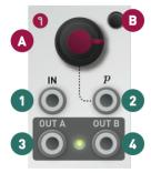
Branches consists of two identical sections called Bernoulli gates. An internal connection routes the input of section 1 to section 2 – unless a jack is connected into the input of section 2.
