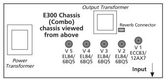
Reverb Connector: red plug: reverb spring input black plug: reverb spring output
