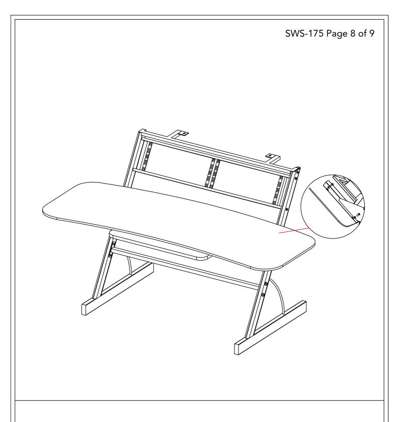
8. Install the main shelf with the wooden screws.
