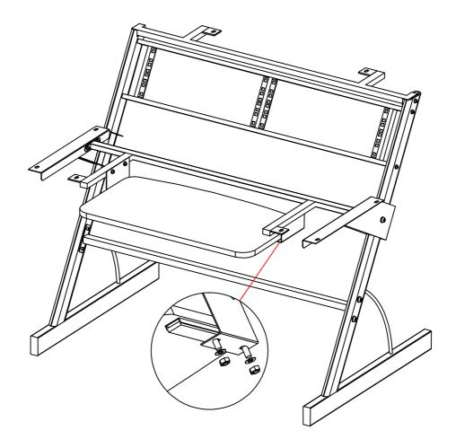
7. Mount the keyboard shelf on the brackets and tighten the screws.
