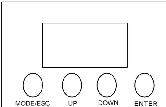
The main menu is accessed by pressing the Mode/Esc-button. Browse through the submenu by pressing Up or Down. Press the Enter-button in order to select the desired menu. You can change the selection by pressing Up or Down. Confirm every selection by pressing the Enter-button. You can leave every mode by pressing the Mode/Esc-button. The functions provided are described in the following sections.
