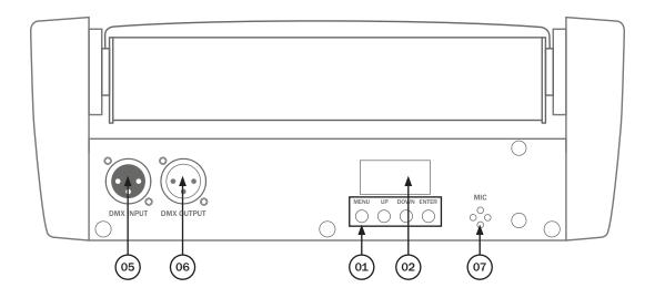
01 - Function buttons 02 - LED display 03 - Fuse F3A 250V 04 - IEC power input 05 - 3-Pin XLR DMX input 06 - 3-Pin XLR DMX output 07 - Microphone 08 - Earth point In the box: 1 x fixture, 1 x hanging bracket, 1 x power cable & 1 x user manual
