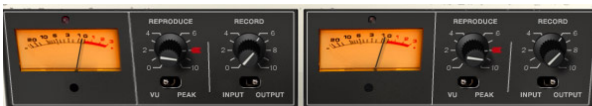
The Ampex ATR-102 “penthouse” showing meters and I/O controls
