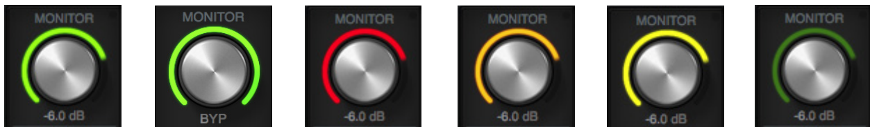
Monitor level indications (from left to right): Normal, Bypass, Mute, ALT 1, ALT 2, and DIM/MONO
