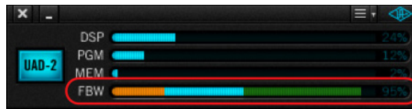
The FireWire Bandwidth meter is visible when a UAD FireWire device is connected
