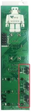
The rear panel of the module features three jumpers that can be used to set the voltage that's passed to the input of each channel when no cable is connected. This feature allows the module to be used as a manually variable voltage without needing to apply any input signal. When the jumper is between the top and middle pin the voltage at the input is 5 V, and when it is between the bottom and middle pin the voltage is 10 V.
