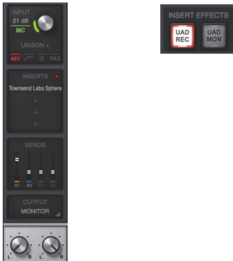
Figure 2-3 Apollo strip with Sphere as first channel insert, 48V active (left); UAD REC button active (right)
