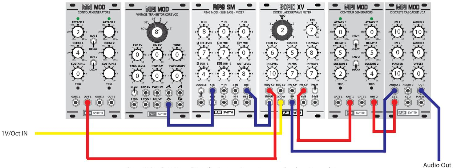
*Note: 1V/Oct for VCO and Gate for Contour Generators are taken from Eurorack Bus
