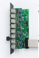
There are 8 jumpers on the FH-1's top PCB, and 1 on the bottom PCB.
