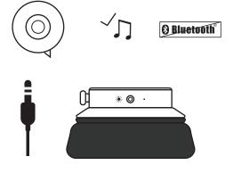
Insert the 3.5mm cable into the port to automatically switch to aux in. HeadSpace does not need to be powered on. If HeadSpace is powered on Bluetooth is disabled to extend battery life.
