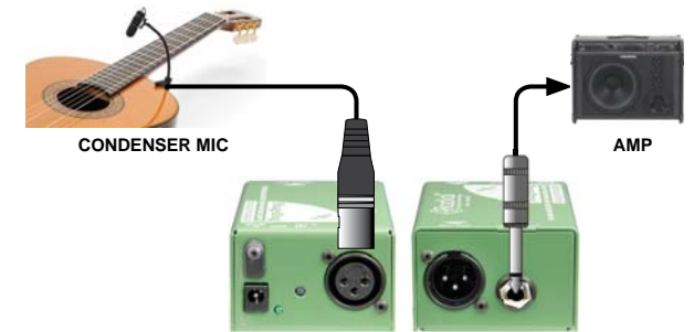
Using the unbalanced 1/4" output with an instrument amplifier.
