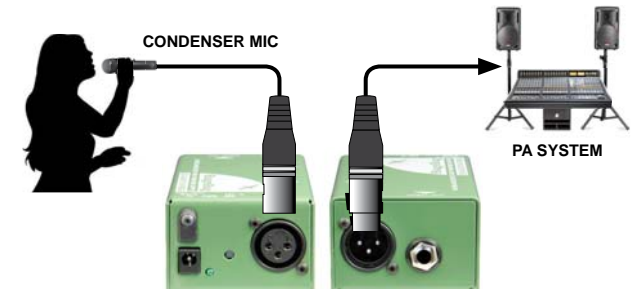
Using the balanced XLR output to feed the PA system.
