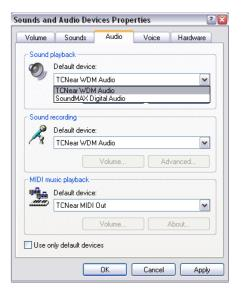
Select "TCNear WDM Audio" for both Sound playback and Sound recording.
