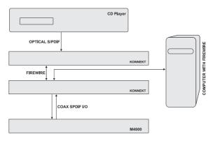
In this setup, we have a CD player in the system. In terms of digital clocking, a CD player cannot be controlled externally and can thus only act as master. Again we have to stress that not only does Studio Konnekt 48 provide a high quality clock, but it also facilitates excellent jitter-elimination that will clean up a less-than-perfect digital signal from an external source such as a CD player.
