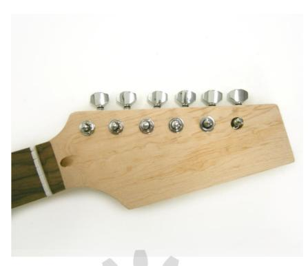
Insert the machine heads (3) in to the holes in the Headstock (2). Place the washer (12) on top, and then screw in the Ferrules (11). The neck should then be turned over and six of the 7mm screws should be screwed in to the pilot holes securing the machine heads in place.
