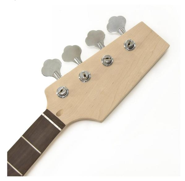
Push the Ferrules (8) into the holes on the front of the Headstock (2). Turn the neck over and screw the machine heads (7) in place using the  $16 \times 7 \text{mm}$  (thin) screws.
