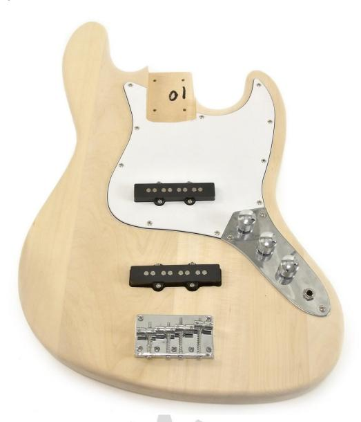
Screw the Bridge pickup back in position. Screw the Tailpiece (5) in to place using the  $7 \times 26$  mm screws and matching the holes in the Tailpiece to the pilot holes. The Control Panel (3) should be attached using the  $3 \times 7$ mm (thick), matching the holes with the pilot holes.
