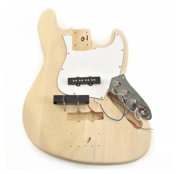
Remove the bridge pickup from the guitar body (1). Feed the blue Earth Wire (4) through the cavity in the body as shown in the picture.
