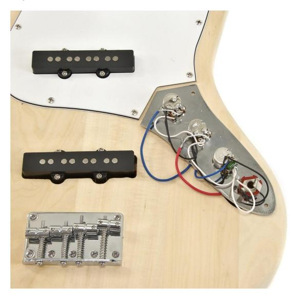
Solder the covered wire from the neck pickup (blue) to the first tone pot arm on the Control Panel (3), and the uncovered wire to the back of the same pot. Solder the covered wire from the bridge pickup (red) to the second tone pot arm on the Control Panel (3), and the uncovered wire to the back of the same pot. Solder the Earth Wire that has been threaded through the body to the back of the Tailpiece (5).
