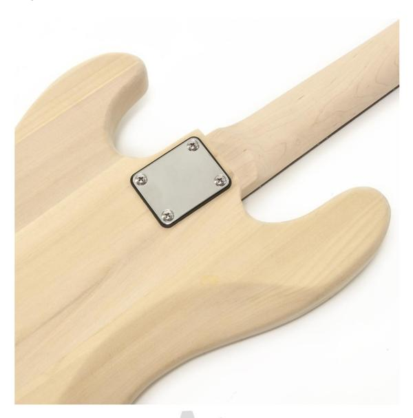
Put the Body (1) and Neck (2) together. Place the Neck Plate (16) with the rubber Padon the back of the Body (1) in line with the pilotholes, and attach with the 4x 45mm screw. Place the Truss Rod Cover (14) in place, matching the holes with the pilot holes, and screw in using the 3 x 8mm (thin) screws.
