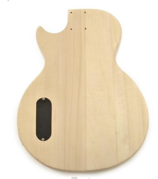
Screw the Backplate (13) in place using two of the 8mm (thick) screws. Turn the Body over and screw the Washers and Nuts from the Tone and Volume knobs to the tops of the Pots that have been inserted through the Body holes.
