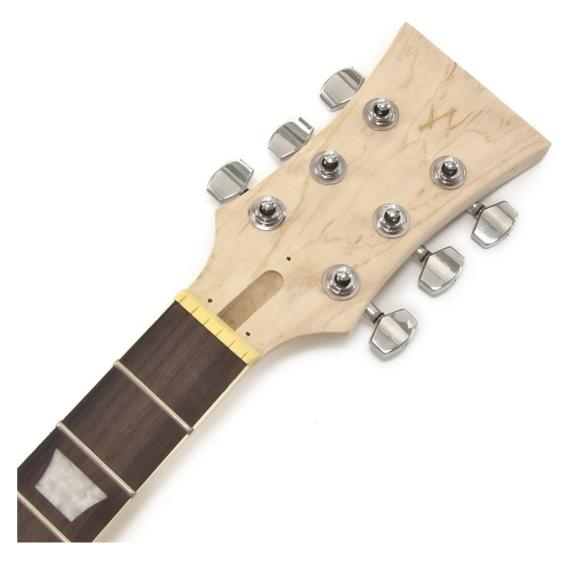
Insert the machine heads (10) in to the holes in the Headstock (2). Place the washer (11) on top, and then screw in the Ferrules (12). The neck should then be turned over and the 6x5mm screws should be screwed in to the pilotholes securing the machine heads in place. Make sure that the screw hole in the Machine Heads are facing downwards.
