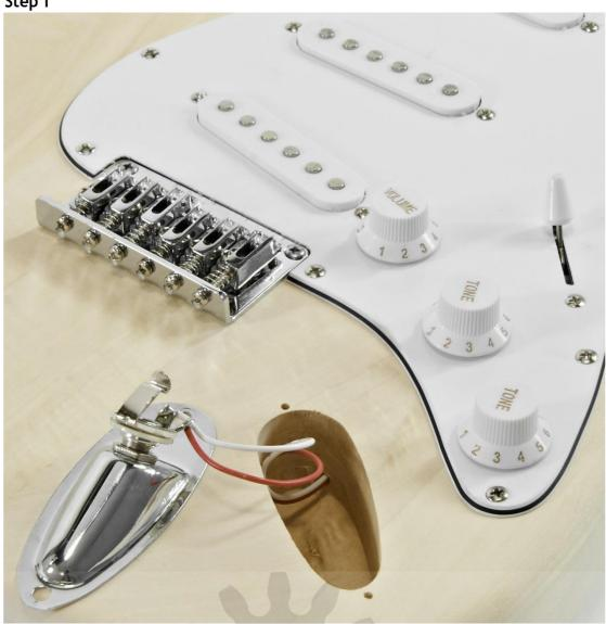
Attach the Jack Plate (4) to the wires coming from the front of the body (1) using the solder provided. The red wire should connect to the longer arm of the jack input, and the white wire to the shorter arm. The Jack Plate (4) should then be placed to match the pilot holes on the front of the body and attached using two of the 6mm screws.
