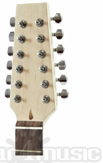
Insert the machine heads (7) in to the holes in the Headstock (3). Place the washer (8) on top, and then screw in the Ferrules (9). The neck should then be turned over and the 7mm screws should be screwed in to the pilot holes securing the machine heads in place.
