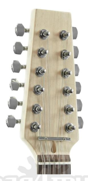
String the guitar with the provided strings (13) and then attach the String Tree (12) to the Headstock (3) using the 9mm screws. The screwshould be placed between the E and A strings on the left hand side of the headstock, and between the B and E strings on the right hand side.
