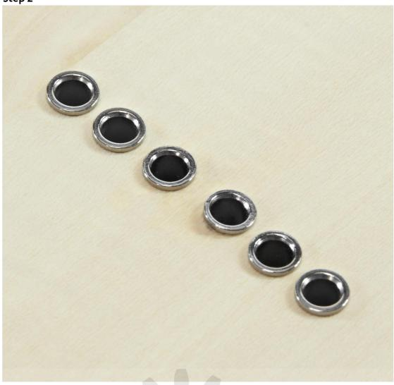
Turn the guitar body (1) over and place the six string ferrules (5) into the holes on the back of the guitar. If the ferrules offer a little resistance, a gentle tap with a hammer can help them into the holes.
