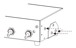
Remove the bolts in the picture on both sides of the TUBE ENGINE to release the rack mounting lugs  $\,$
