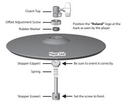
Orient the stopper (upper) so that it matches the groove in the hi-hat.
