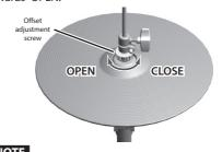
If the sound cuts off when you strike the hi-hat forcefully, rotate the VH offset adjustment screw towards "OPEN."
