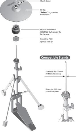
\* When turning the VH-10 upside down, protect the clutch and the sensor from damage. Handle the unit with care so that it is not
