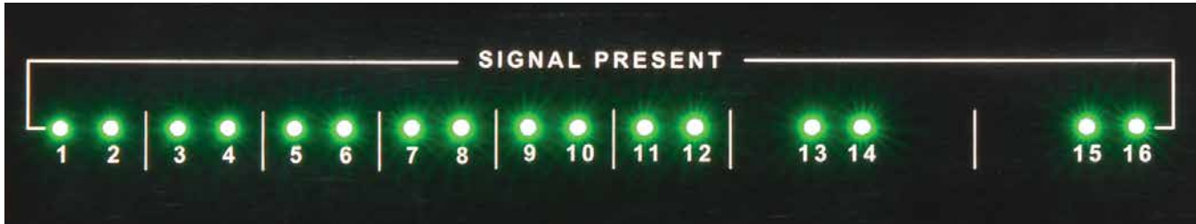
[SIGNAL PRESENT LEDS PICTURED ABOVE]
