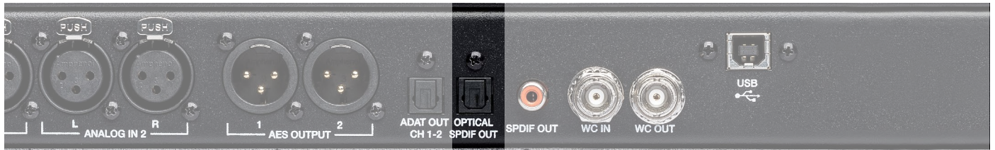
[REAR PANEL SPDIF OPTICAL OUTPUT CONNECTOR PICTURED ABOVE]
