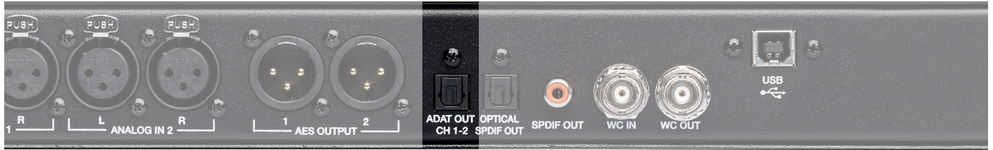
[REAR PANEL ADAT OPTICAL OUTPUT CONNECTOR PICTURED ABOVE]
