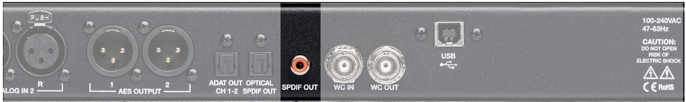
[REAR PANEL SPDIF COAXIAL OUTPUT CONNECTOR PICTURED ABOVE]
