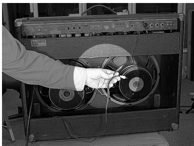
Some amps have jacks on the chassis to disconnect the reverb tank RCA cables.
