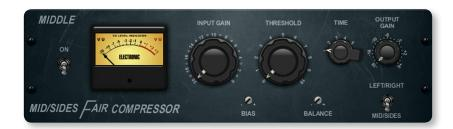
The Fairchild 670 tube compressor not only achieves record bids in high-end vintage gear auctions, it also delivers some of the finest colorations in compressor history. Two small trim VR's preset the control side chain action, a six-step switch determines the timing, and the two large Input and Threshold knobs adjust the levels.
