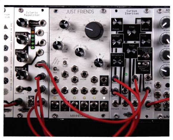
Dynamically generated wavetable oscillator using orthogonal functions.
