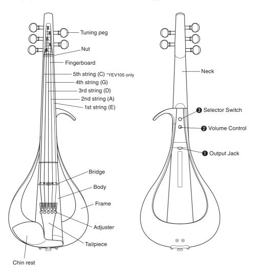
The YEV105 (5-string model) is used in the illustration. The number of strings/tuners, and the shape of the fingerboard and tailpiece are different on the YEV104 (4-string model).
