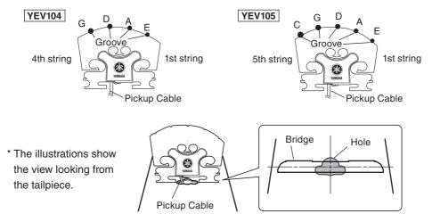
• Ensure that the bridge stands vertically. If it leans to one side, use both hands to adjust. Make sure that each string passes over the corresponding slits in the bridge.
