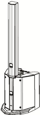
In the collapsed position, you do not use the speaker extension as shown in the example to the left.
