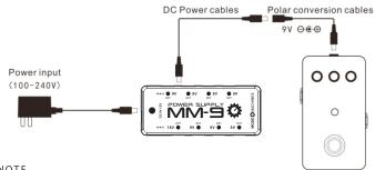
Before use, please confirm the equipment is the same polarity with the power adapter, otherwise may cause damage
