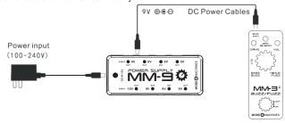
If the input polarity of the electrical device is  $\bigcirc$   $\bigcirc$   $\bigcirc$  please connect polarity reversal cable to the DC power cable, then connect the device
