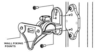
Fit the Wall bracket to the spacer as shown with M3 screws included.
