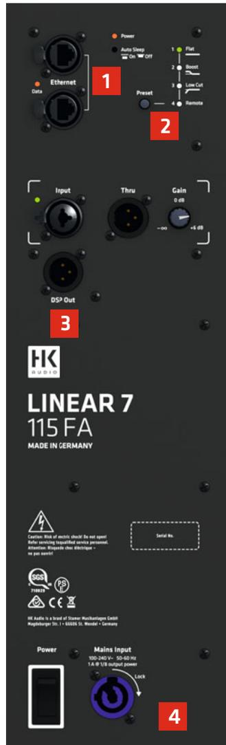
**1** All models in the LINEAR 7 family feature analog balanced inputs and outputs as well as professional Ethercon ports. And all devices in the system can be daisy-chained if required – that is, connected in series.
