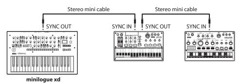
Use the same settings for "Sync Out Unit" (p.44) on this minilogue xd and "Sync In Unit" on the first external device to sync. Similarly, use the same settings for "Sync In Unit" on the second external device to sync.
