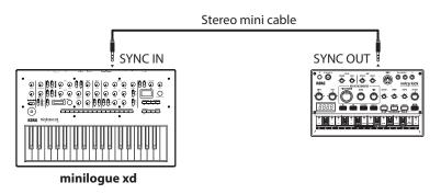
Use the same settings for "Sync In Unit" (p.44) on this minilogue xd and "Sync Out Unit" on the external device. Similarly, use the same settings for both the "Sync In Polarity" (p.44) and the "Sync Out Polarity" on the external device.
