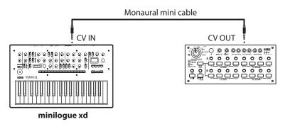
Configure the CV IN jack settings on the minilogue xd from "Button 5 (CV INPUT)" (p.36). See the owner's manuals of each respective external device to synchronize.
