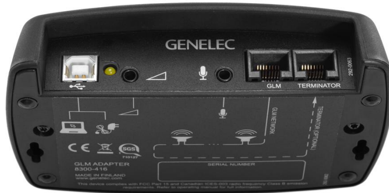
Figure 37. GLM Network Adapter connections from left to right, USB to computer or to USB power supply, hardware level controller input, GLM measurement microphone input, GLM network and terminator connectors.
