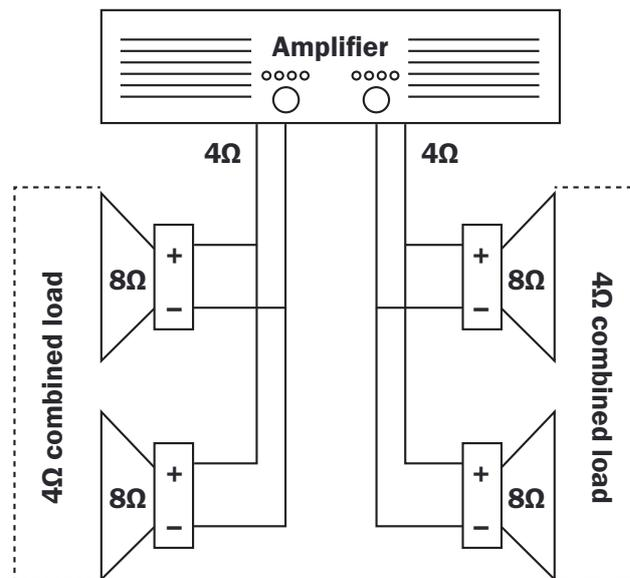
Series parallel 4 loudspeaker mono setup
