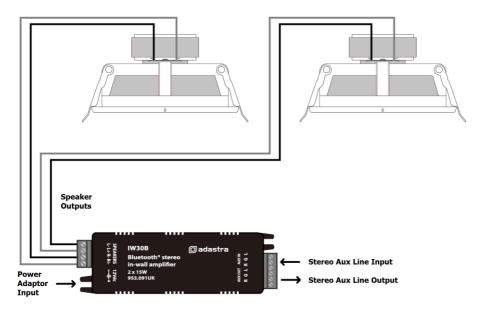
Connect speakers using the supplied wires or equivalent by connecting "+" and "-" on the speaker to the relevant connection on the amplifier. The speaker connections are via screw terminals on a Euroblock, which can be removed for easy access whilst making connections. Once connected, install each speaker by bending the spring clips back, feeding the speaker into its cut-out in the wall or ceiling and releasing the springs to clamp it in place.
