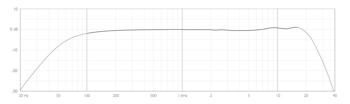
Typical on-axis frequency response of 2028 Vocal Microphone measured at 12 cm (4.7 in).
