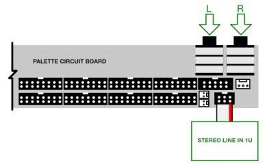
**IMPORTANT**: If you connect a module to the Audio Jacks Connector, you should not connect a module to the Link Connector (described below). Since both connectors access the Audio Jacks on your Palette case, unexpected results may occur.
