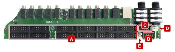
Running along the back edge of the Pallette is its built-in circuit board, which contains all of Palette's audio, midi, power, and module connection circuitry.
