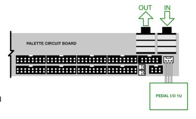
**IMPORTANT**: If you connect a module to the Links Connector, you should not connect a module to the Audio Jacks Connector (described previously). Since both connectors access the Audio Jacks on your Palette case, unexpected results may occur.
