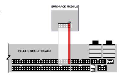
Plug the other end of the ribbon cables into the Eurorack modules you wish to power — being careful (if the module's power connector isn't shrouded) to align the red stripe with the -12V pins on the module. These pins are indicated differently by different manufacturers, but often will say "-12V," or "Red Stripe," or have a visible white stripe next to the -12V side of the connector. See your Eurorack modules for details concerning its -12V power nomenclature.
