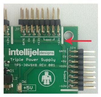
The other end of the cable, with a 16-pin connector, connects to the power bus board of your Eurorack case. Ensure the red stripe on the cable lines up with the -12V pins on the bus board. On Intellijel power supplies the pins are labelled with "-12V" and a thick white stripe.
