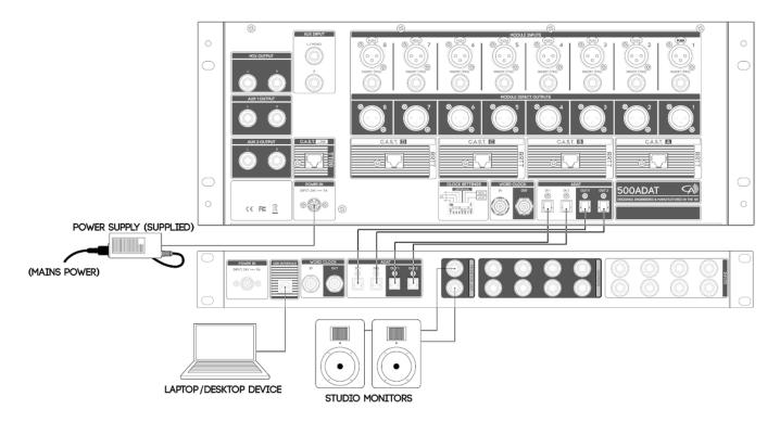
This hardware setup diagram will get 500ADAT connected to your audio interface and ready for recording.
