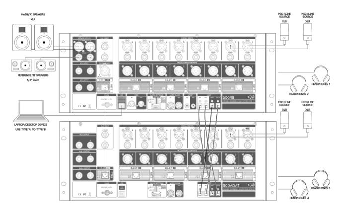
Each unit features 2 ADAT IN and 2 ADAT OUT ports that can be used to achieve 8 channels of expansion from 44.1kHz to 96kHz. When the two units are connected, you are able to patch to and from 500ADAT by using the ADAT I/O from within your DAW I/O routing.
