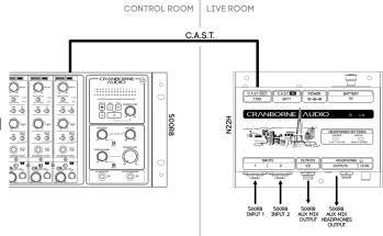
DC power supply or via an internal 9v battery. Power is only drawn when the headphone output has been plugged-in to preserve battery life and when the headphone amp is not required, you can simply use the combi jack inputs as passive input connections.
