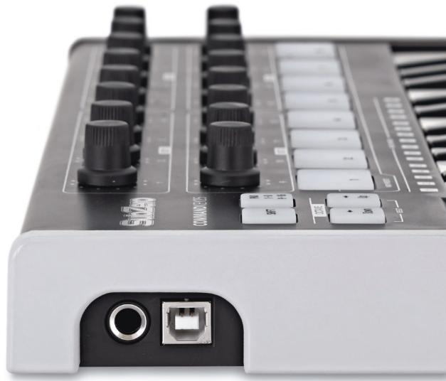
The footswitch jack functions as an on/off switch and can be configured for either momentary applications (such as sustain pedal) or latching behaviour (first press/release sends one event, second press/release sends the next event).
