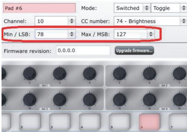
The first press of Pad 6 will send a CC# 74 command with a value of 78, which will close the filter down part way but still let a lot of the audio pass through. The second press of Pad 6 will send a value of 127, opening the filter completely.
