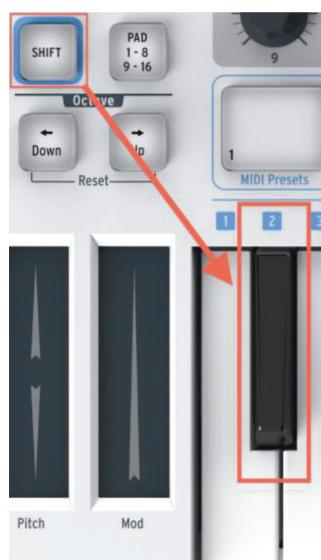
Then when it's time to switch to channel 1, for example, use the same technique but press a different key: in that case, you would hold the Shift button and press the first C key on the keyboard.
