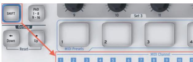
The numbers above the first 16 keys on the keyboard correspond to the 16 possible MIDI channel numbers, and indicate which key you should use in conjunction with the Shift button to change the Global MIDI Channel setting. For example, if you want to switch the Global channel of the COMMANDKEY to MIDI Channel 2, hold the Shift button and press the first C# key:
