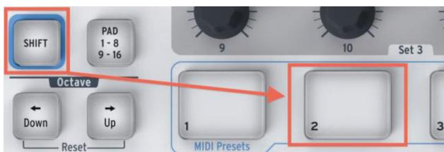
In the picture above, the combination of the Shift button and Pad 2 will select Preset #2 from the COMMANDKEY preset memory locations.
