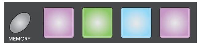
The combination of the Memory button and pad 2 will recall preset #2 from the CONTROLPAD64's memory.
