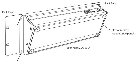
Use existing screws x 4 and tighten the Rack Ears securely to the synthesizer
