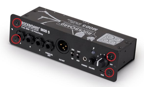
Remove the screws as indicated below to release the front plate from your MOD 5 using a PH2 Phillips head screw driver. The mounting nuts of the jack sockets do not have to be removed!
