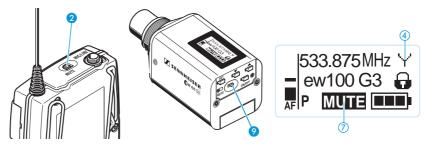
The MUTE switch ② (SK)/ ③ (SKP) allows you to mute the audio signal or to deactivate the RF signal. Via the "Mute Mode" menu item, you can set the desired function of the MUTE switch ② (SK)/ ③ (SKP):
