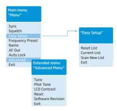
When one of the standard displays is shown on the display panel, you can get into the main menu by pressing the SET button 3. The extended menu "Advanced Menu" and the "Easy Setup" menu can be accessed via the corresponding menu items.
