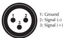
DMX-input XLR mounting-plug:
