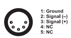
DMX-input XLR mounting-plug:
