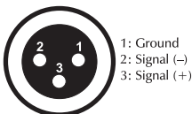
DMX-output XLR mounting-socket:
