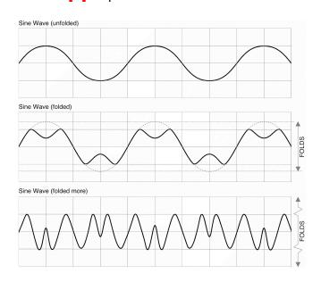
Any modulation applied to the FOLD P [G] or FOLD S [H] CV inputs varies the amount of folding around the value set by the FOLD knob, with positive CV increasing the amount of folding applied by the respective (P or S) circuit, and negative values decreasing it.
