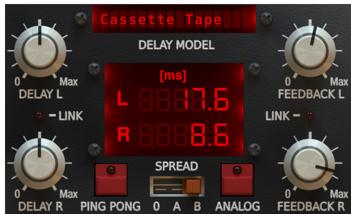
Repeater delay line parameter control section
