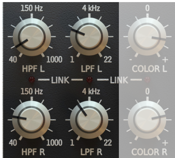
Filter cut-off frequencies for both stereo channels
