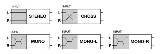
Stereo ......Inputs are routed to the same delay lines (R to R and L to L). *Cross* ......Inputs are routed to the other delay lines (R to L and L to R). *Mono* .....Inputs are summed and routed to both delay lines. *Mono-L*.....Inputs are summed and sent to the left delay line only. *Mono-R* .....Inputs are summed and sent to the right delay line only.
